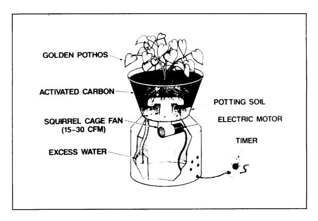
Figure 1. Indoor air purification system combining houseplants and activated carbon.
