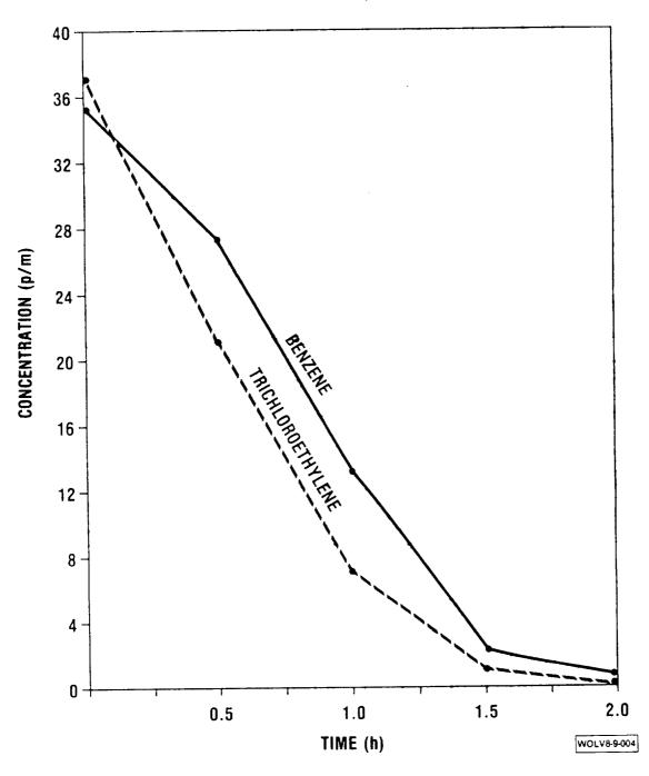
Figure 4. Removal of high concentrations of benzene and trichloroethylene from the air inside sealed experimental chambers using golden pothos in an 8-in. activated carbon filter system.
